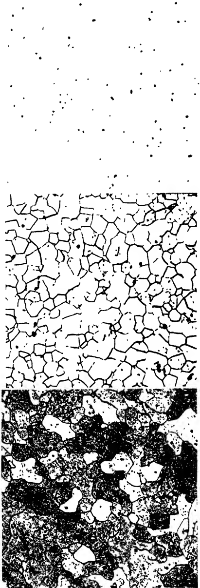
FIGURE 37. Stages in the etching of a metallographic specimen of commercially pure ingot iron. a. (Top) Specimen “as polished.” Dark spots are largely oxide inclusions. b. (Middle) Polished specimen after light etch. Dark lines are grain boundaries. c. (Bottom) Polished specimen after heavy or contrast etch. All grains have essentially the same composition but etch at different rates because of differences in orientation.
